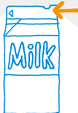
Semicircular cutout on the opposite side of the pour spout of milk cartons
